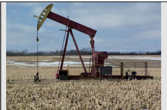
Typical oil well with pumping unit
